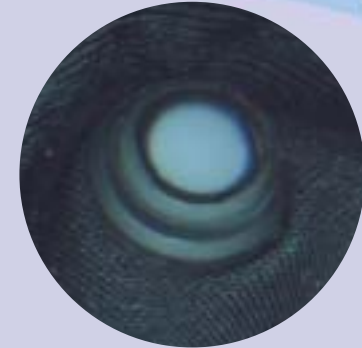
Close-up of electrode cup shows reservoir with gel.
