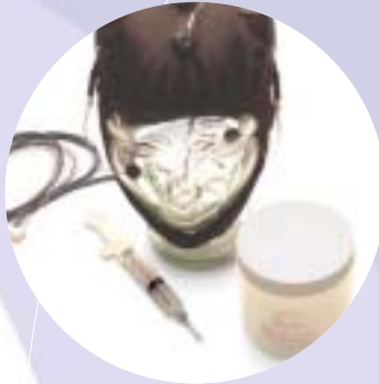
Only conductive gel and a blunt-tip syringe are required for fast set-up.
