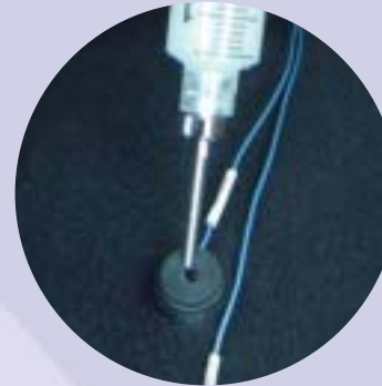
Unique blunt tip delivery helps part hair and obtain good impedance values.
